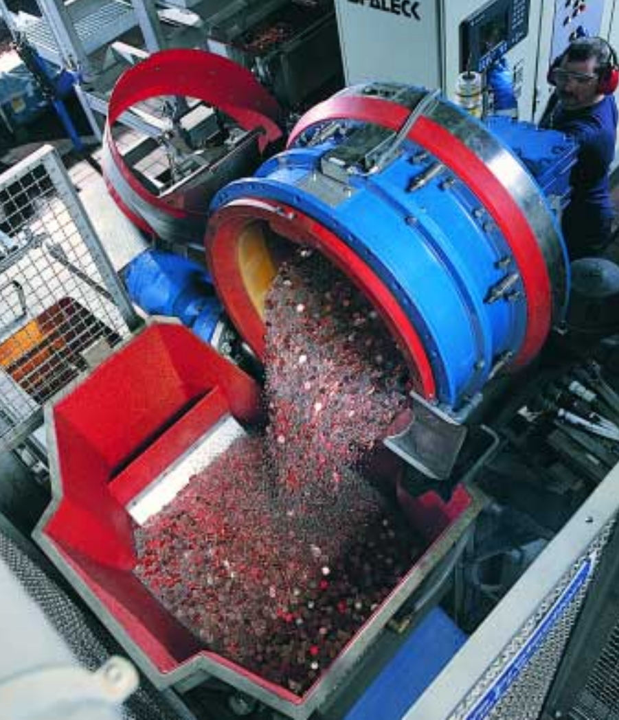
A new high energy burnishing machine, installed to improve the quality of blanks. (Molyneux Associates)
