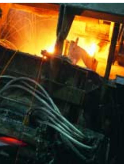
Above: Molten nordic gold, the chosen alloy for the 10, 20 and 50 euro cent coins, being transferred into the holding furnace prior to casting. (Molyneux Associates)
